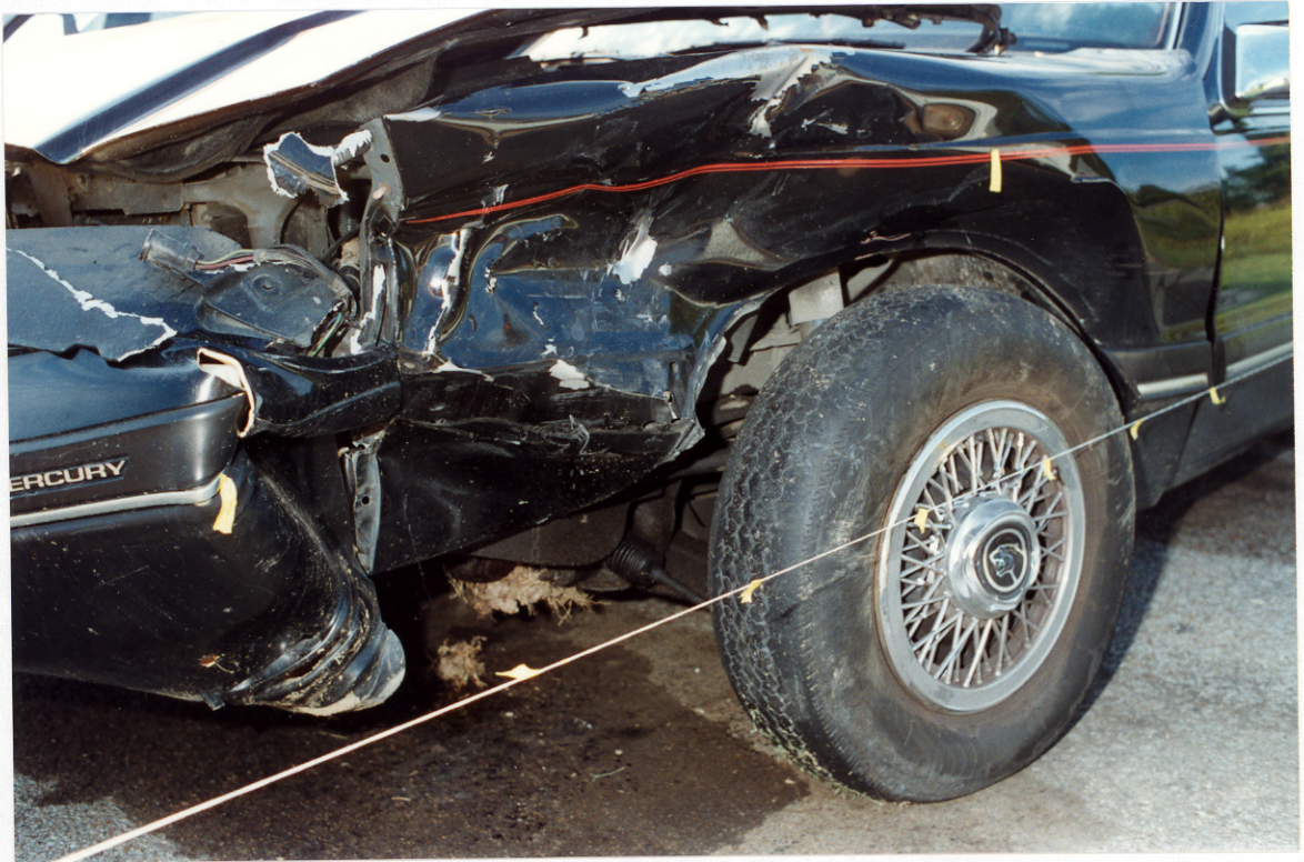
107. Close-up view of the direct contact damage.
